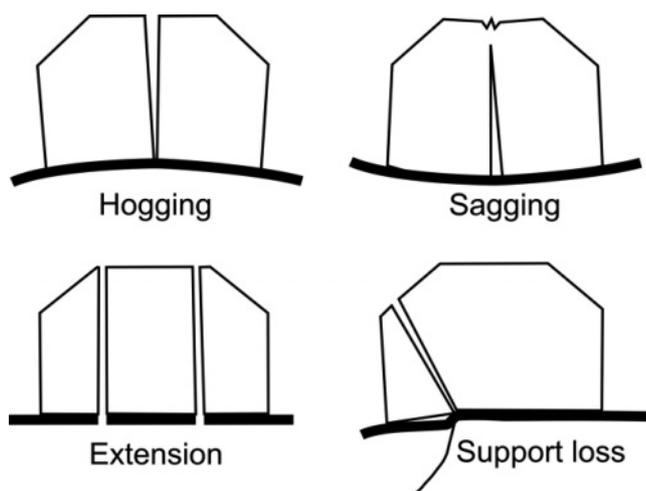
**Fig. 1.** Schematic illustration of building damage associated with various types of subsidence movement, some of which may occur together. In practice, these movements are concentrated in areas such as windows and doors, and may occur in many places throughout the building.
