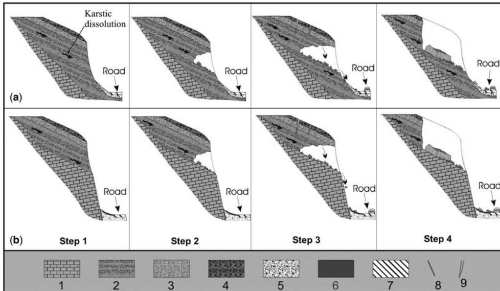
**Fig. 12.** Phases of cave evolution (a) along a talus slope and (b) along the contact between inclined talus and limestone: 1, carbonate bedrock; 2, incoherent or partially incoherent debris; 3, coherent debris; 4, soil; 5, talus; 6, fall deposits and soil; 7, anthropic deposits; 8, fault; and 9, fracture.
